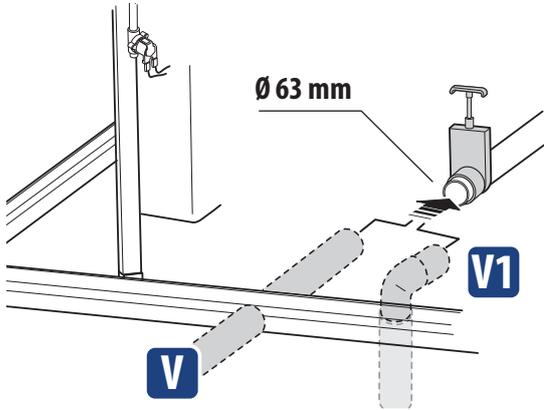
**Note on connecting the balance tank drain:** the factory installed pipe is fitted with a connector with gaskets, which the drainage system in the building can be connected to. Alternatively, the balance tank can be connected directly to the drain (remove the factory installed pipe) and the connector supplied (or a valve) can be used to drain the water as necessary.
