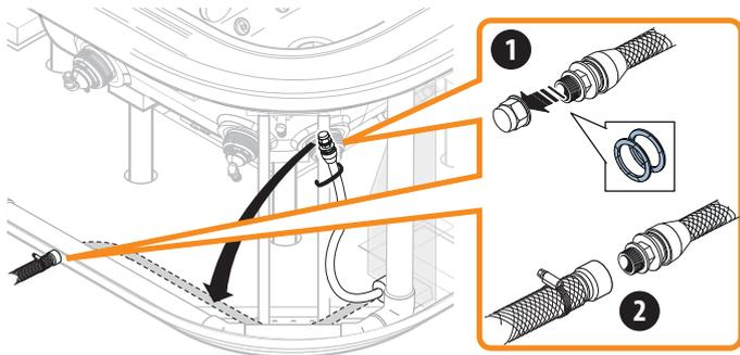
► Connect the solenoid valve to the water mains.
